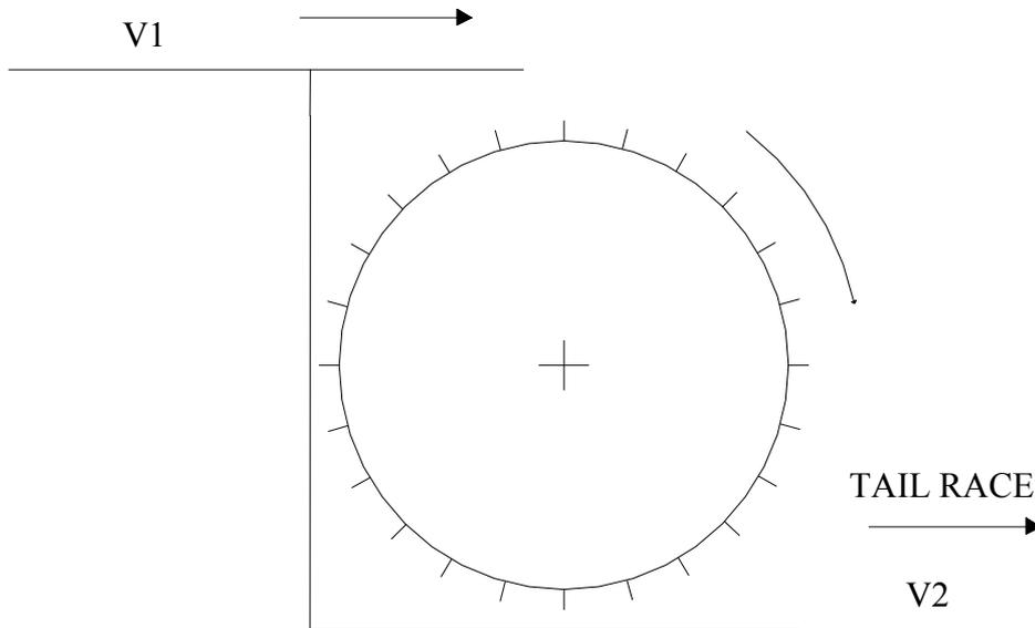
In the overshot wheel we must consider the kinetic energy of the flowing water as well as the potential energy provided by the height difference between the head race and the tail race. In essence we are applying the energy equation which is another way of expressing the conservation of energy.
