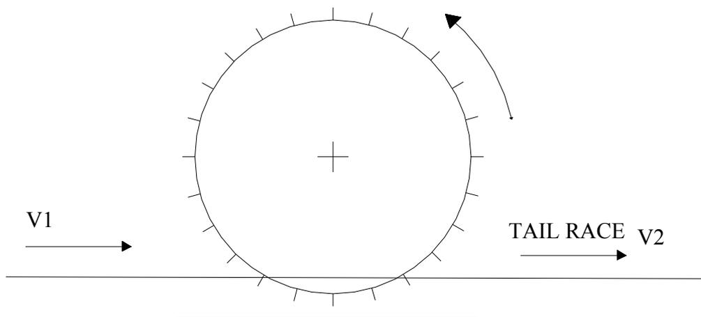
The volume of water hitting the blades is dependent upon the speed in the flume  $V_1$ ; most treatments work out the volume then multiply by this speed to give a volume then a weight. Here I shall nominate  $W$  for the weight generated by the speed of the water flow, it is the same thing.
